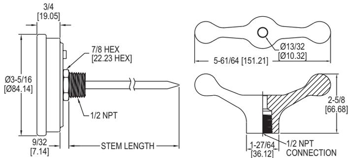
The **Series BTLRN Long Reach Bimetal Thermometer** reaches areas that other thermometers can't. A gripping handle is available as an accessory to comfortably hold the thermometer during temporary installations.
