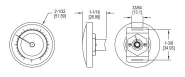
The **Series BTP Pipe-Mount Bimetal Surface Thermometer** is designed to accurately measure the surface temperature of a pipe.
