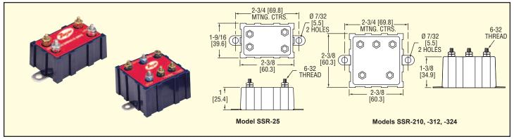
Series SSR Solid State Relays amplify the current handling capability of a variety of sensors for controlling higher power loads. The relays are compact, totally encapsulated and impervious to shock or vibration. Units feature SPST, normally open switch operation and can control loads up to 5A or 10A depending on model.
