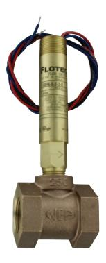
The Series V6 FLOTECT® Flow Switch is an inexpensive, explosion-proof flow switch for use on air, water or other compatible gases and liquids. Three configurations are available - 1. Factory installed in a tee. 2. With a trimmable vane for field adjustment and installation in a suitable tee. 3. Low flow models with an integral tee and adjustable valve. All are available with an optional enclosure which is UL and CSA listed, or Directive 2014/34/EU (ATEX) compliant for
