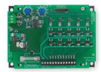
The Series DCT500ADC Low Cost Timer Controller is designed to provide continuous or on-demand cleaning for 10-35 V powered receivers and pulse jet systems. It is available in either 4, 6, or 10 channels, and each unit is the same size, minimizing enclosure space and reducing overall system installation cost. For added safety, the control circuitry including the control inputs are isolated from the line voltage.
